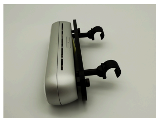
(b) Part 3 screwed to D455 camera.
